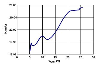
FIGURE 4. LOAD REGULATION  $(V_{IN} = 4V)$
