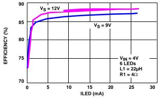
FIGURE 8. EFFICIENCY IMPROVEMENT WITH 9V AND 12V INPUTS
