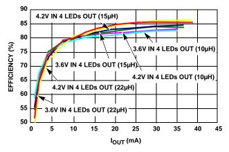
FIGURE 2. EFFICIENCY vs LED CURRENT
